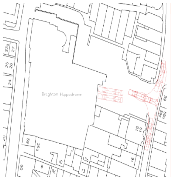
Figure 10: Illustration of access to the rear of the theatre for 16.5 m artic
